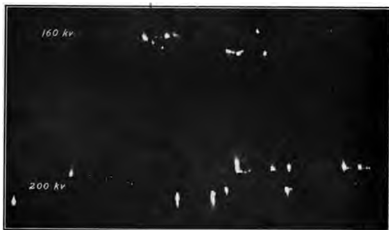
FIG. 68.—Corona on a No. 3/0 line cable. Wet. (Facing page 75.)
